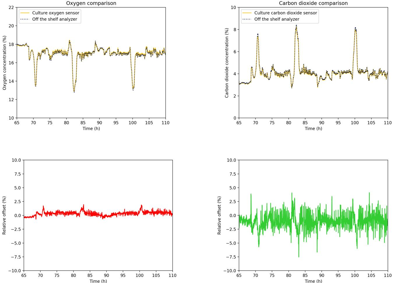
Figure 3. O2 and CO2 concentration of live yeast fermentations recorded by Culture Bioscience's off-gas analyzer and a commercially available off-gas analyzer. The relative percent offset from the Culture sensor and the off the shelf unit are plotted in the second row.
