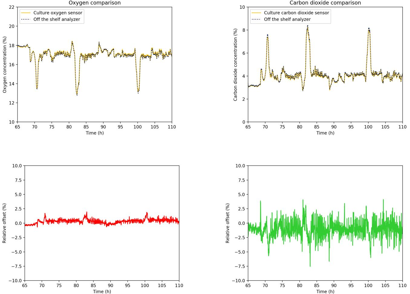
The results of this comparison show that Culture Bioscience's off-gas analyzer behaves almost identically to the off the shelf analyzer when used in a typical fermentation process (i.e. typical aeration rate and headspace containing water vapor, volatile metabolites, etc.).
