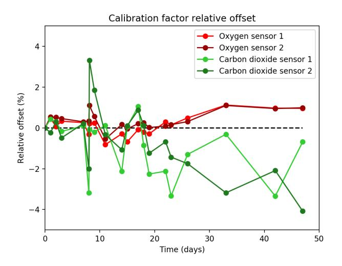
**Figure 1.** Relative drift of two  $O_2$  and two  $CO_2$  sensors over 40+ days while running continuously in active microbial fermentations.
